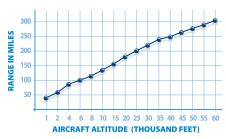
Optimal Line-of-Sight (LOS) transmission distances relative to aircraft altitude on a clear night with low humidity, over flat terrain.
