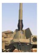
**UBS-6G** Universal Base/Spring assembly for VCF antenna family, with integrated high gain GPS antenna, LNA and filter.
