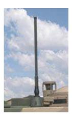
VCF136-174 136-174MHz Mobile VHF Comercial Band (LMR), Center-fed Dipole Antenna
