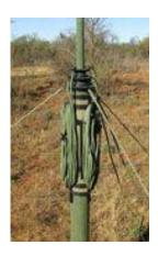
**RTM-8**8 Meter Telescopic Mast for small to medium sized antennas in static mobile and base station communication applications.
