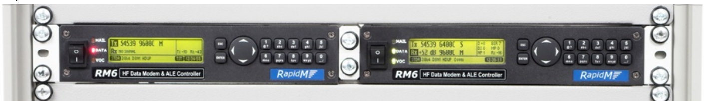
Fig 2: Two RM6 Units side-by-side in a 19-inch rack
