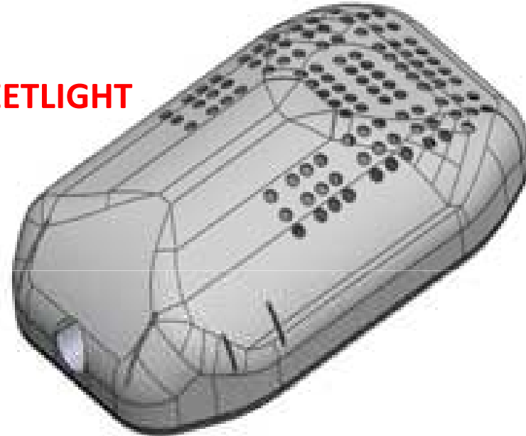
Thermal Management :Heat sink
